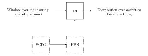
Fig. 1. System flow chart. Dashed lines indicate off-line components and solid lines indicate online components. Level 1 action symbols and the HBN are merged via the deleted interpolation step to produce level 2 actions.
